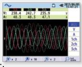
**Harmonic Analysis** Read harmonic components of voltage and current per CH with a colored graph
