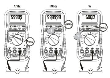
**Note:** Unlike the Line Level Frequency measuring function as previously stated, this Logic Level Frequency function is set only at the highest input sensitivity for measuring digital type electronic signals.
