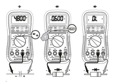
Normal forward voltage drop (forward biased) for a good silicon diode is between 0.400V to 0.900V. A reading higher than that indicates a leaky diode (defective). A zero reading indicates a shorted diode (defective). An OL indicates an open diode (defective). Reverse the test leads connections (reverse biased) across the diode. The digital display shows OL if the diode is good. Any other readings indicate the diode is resistive or shorted (defective).
