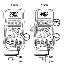
Note: Be sure to insert the banana plug K-type temperature bead probe Bkp60 with correct + → polarities.
