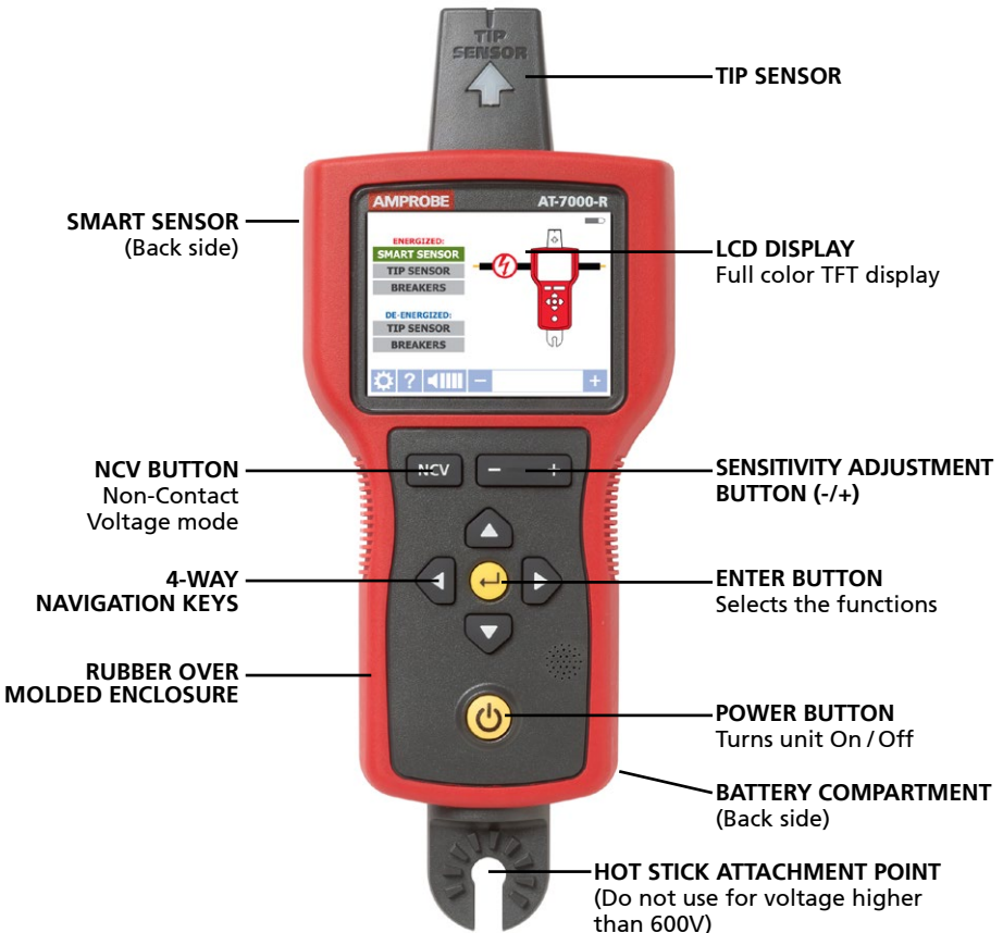
Figure 1: Overview of AT-7000-R Receiver
