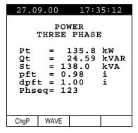
Example of screen in "4 wires" three-phase mode
