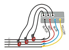
Instrument connection in a three-phase 4 wire system
