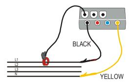
Instrument connection in a single-phase system
