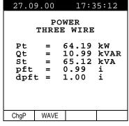
Example of screen in "3 wires" three-phase mode
