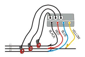
Instrument connection in a 3 wires three-phase system
