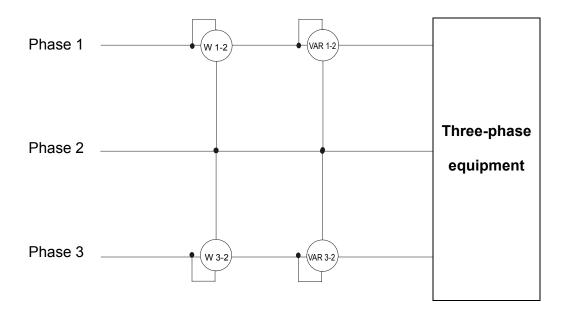
In this case the potential of one of the three phases (for example, phase 2) is taken on as reference potential. The total values of the active, reactive and apparent power are expressed as sum of the indications of the couples of Wattmeters, VARmeters and VAmeters.
