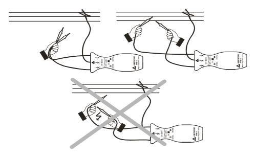
Check for voltage on all phases: three LEDs marked "A", "B" & "C" should be on. If there is a lack of voltage on one of the test leads the corresponding LED will not illuminate. If a voltage is pre-
